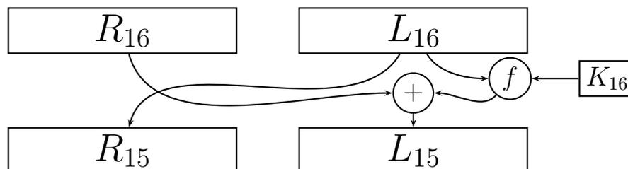
In other words, to decrypt a message, you may use the same mechanism that was used to encrypt, except apply the Key Schedule in reverse, meaning first use  $K_{16}$ , then  $K_{15}$ , and so on. This explains why  $L_{16}$  and  $R_{16}$  were reversed at the end of the encrypting process.
