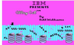
For these computers, a pixel on the television screen represented two bits and there were four colors because each two bit combination, 00, 01, 10 or 11, could represent a different color.
