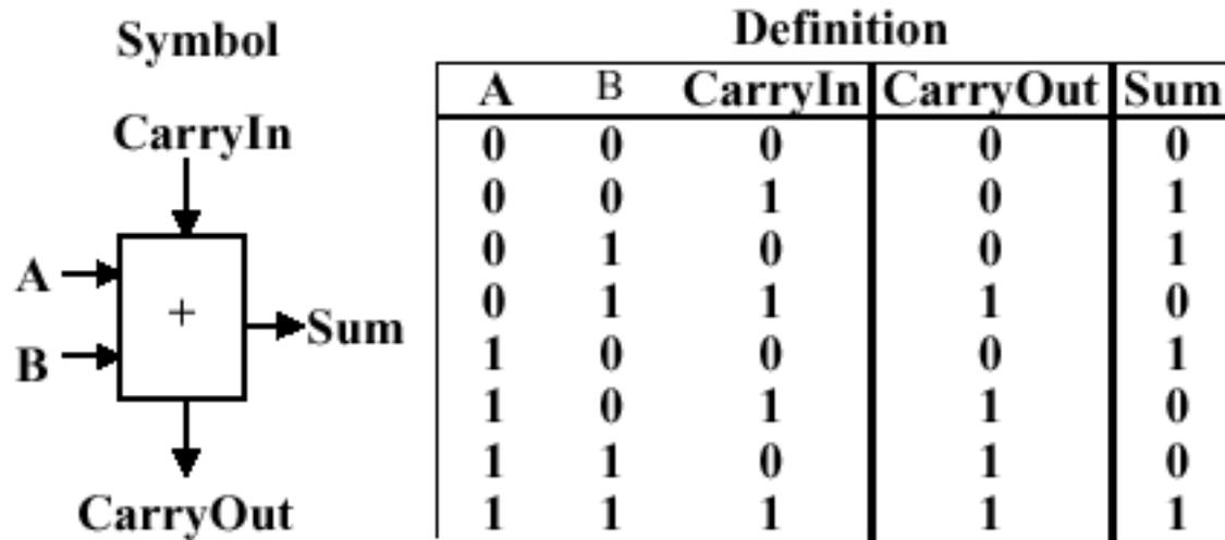
$$\begin{aligned} \text{CarryOut} &= (A*B*CarryIn) + (A*B*CarryIn) + (A*B*CarryIn) + (A*B*CarryIn) \\ &= (B*CarryIn) + (A*CarryIn) + (A*B) \end{aligned}$$
