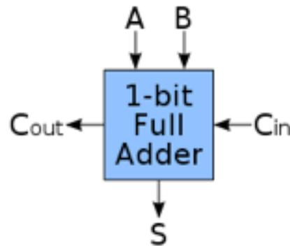
Schematic symbol for a 1-bit full adder with  $C_{in}$  and  $C_{out}$  drawn on sides of block to emphasize their use in a multi-bit adder
